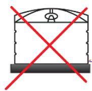
Unsupported pipework or no flexible section.
